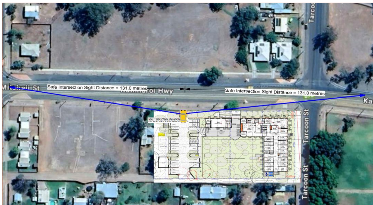
Figure 4: Sight Distance Requirements at Access Driveways Under Austroads Guide to Road Design – Part 4a
